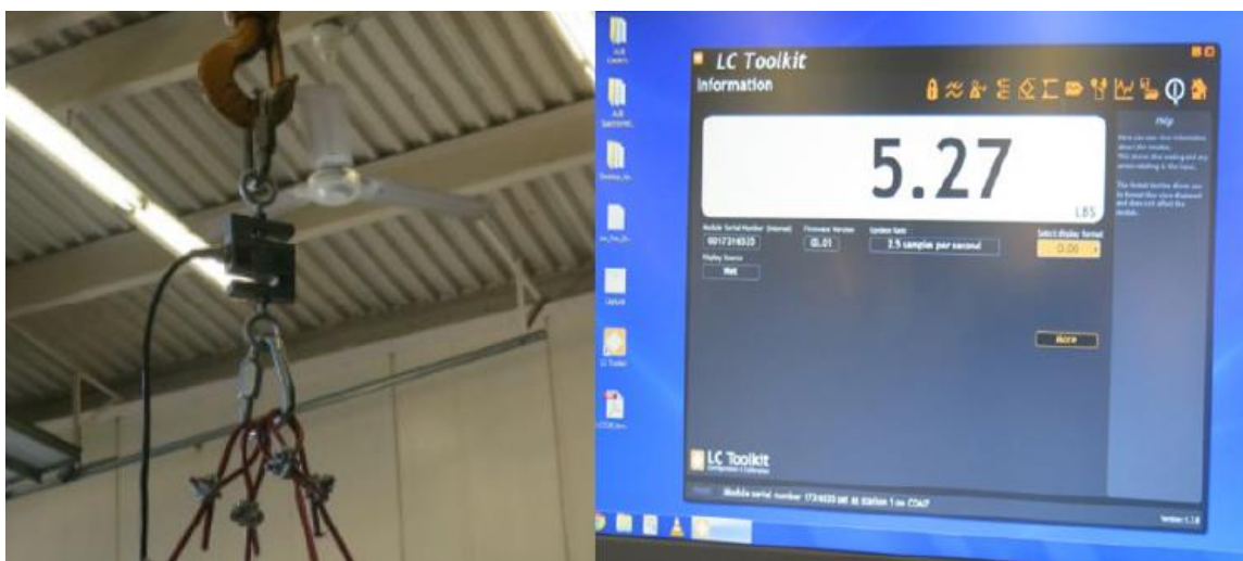
Figure 6. Left: Hoist-mounted load cell read-out configuration for raising/lowering the support rack. Right: Digital read-out display.
