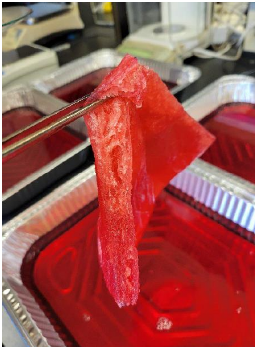
Figure 26. Imbiber Fiber™ sample experiencing delamination at 24-hour mark of ASTM F726-17 test with diesel fuel.
